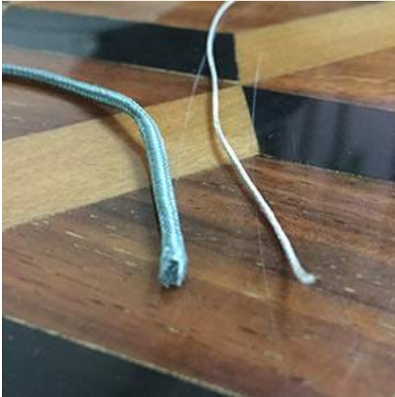
The tubular structure of hollow braid versus the multi stand non-spliceable braided line viewed from the front.
